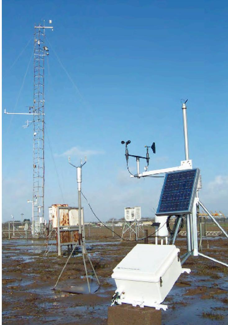
**Fig. 3: Prototype WIRS installed adjacent to UCD/NOAA Climate Station (in background).**
