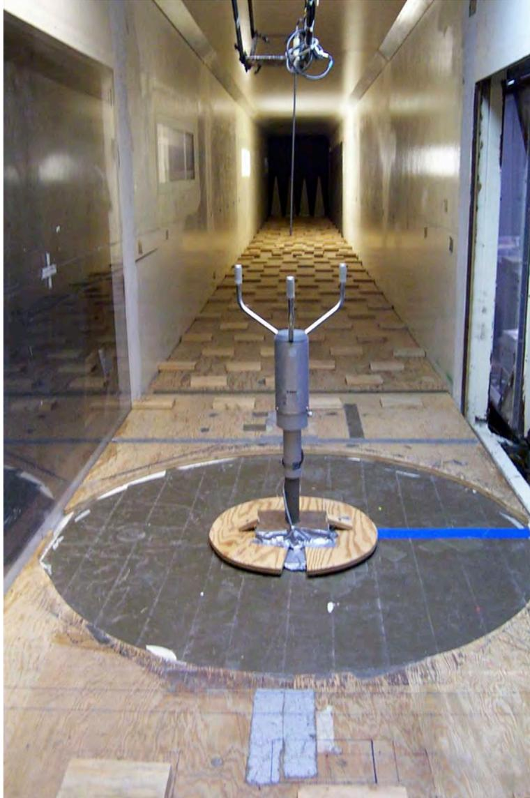
**Fig. 6: Wind tunnel test of Vaisala sonic anemometer**
